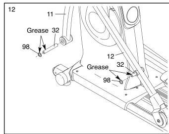
13. Orient the Left Pedal Leg (14) as shown, and slide it onto the Pedal Leg Axles (32). Attach the Left Pedal Leg to the Left Handlebar Leg (11) with two M10 x 20mm Patch Screws (91), two Axle Caps (31), and two M10 x 25mm Washers (94).
